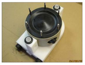
**Fig 22.** Put on the inlet and outlet connections (13), make sure all o-rings (18) are mounted.
