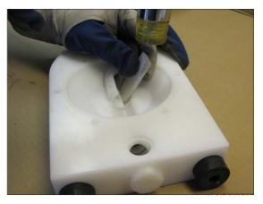
**Fig 2.** To remove the spacer sleeve (19), use a piece of plastic and a hammer to carefully knock to turn it.
