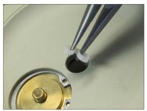
**Fig 10.** To mount the shaft seal (36), bend it to a kidney shape and insert carefully to the groove.
