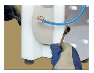
**Fig 24.** Fasten the nuts (37) alternatingly, with or without washers depending on how much of the thread comes out. If some of the nuts were fastened without washer, unscrew thoose and put washers underneath. Tighten the nuts according to recommended tightening torques in chapter 5.
