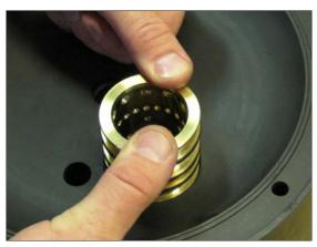
**Fig 6.** Make sure all four o-rings (pos 30) are mounted on the cylinder. Use a little water on the o-rings to easier slide the cylinder into the centerblock. Other lubricants should not be used.
