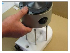
**Fig 20.** Make sure all pin screws (14) have one nut (37) and one washer (38) each. Nut should only be put on one or two threads. Put the pin screws through the housing and the stainless steel side plate and mount carefully the center block assembly.
