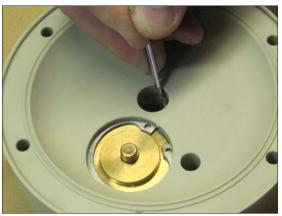
Fig 10. If the shaft sealings (36) seem to be worn out (by internal leakage of air), carefully remove them with a pointed tool. During this operation, the sealing (36) and backup o-ring (47) usually get destroyed, so make sure to have replacement spares available.
