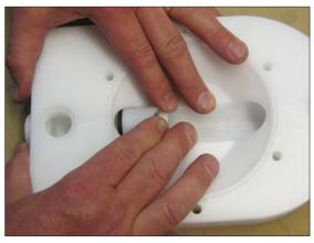
Fig 14. Push the lower valve seat assembly into the housing (11)
