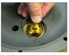
Fig 7. Place the last o-ring (pos 30) on the cylinder.
