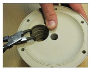
Fig 1. Mount the circlip (27) on one side.
