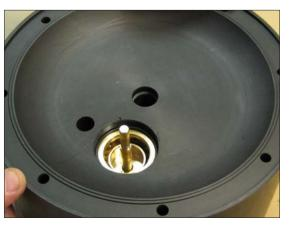
**Fig 14.** Now when both endcaps are removed, push out by hand the shaft and piston.
