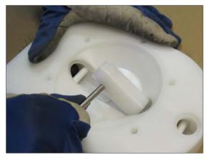
**Fig 4.** Carefully pull out the spacer sleeve (19). Please note that force never shall be used for dismantling.
