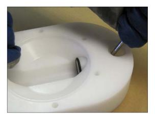
**Fig 6.** Push out the upper valve seat (20), be careful not to damage the edge of the connection hole.
