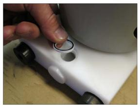
**Fig 21.** Put the small o-ring (pos 18) in the seat of the housing. On pumps with PTFE diaphragms the PTFE u-ring with its o-ring shall be mounted with o-ring facing upwards (see Fig. 21).
