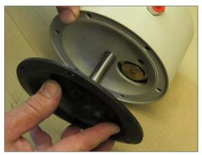
Fig 12. Mount the diaphragm shaft (16) on the diaphragm (15) and push the assembly carefully through the hole in the centerblock (12).
