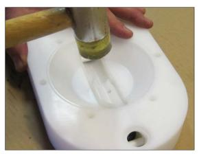
**Fig 18.** Make sure the seat and sleeve assembly is flat inside the housing.
