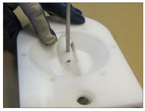
Fig 3. Put one of the pin screws in the hole of the spacer sleeve (19) and turn it all the way  $180^{\circ}$ .
