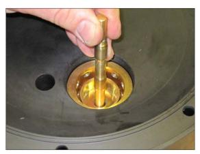
**Fig 8.** Carefully mount the piston and shaft by hand. Repeat steps Fig 3 and Fig 4 on the remaining side. Carefully secure the endcaps equally on both sides.
