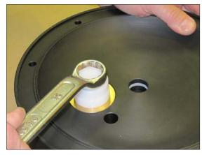
**Fig 4.** Tighten carefully by means of the mounting tool (pos 282) and a spanner.
