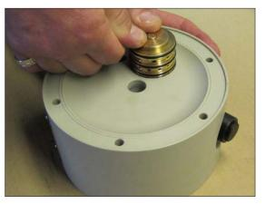
**Fig 2.** Put a little water on the o-rings (30), other lubricants should not be used. Carefully push the air valve (61) into the housing. Mount the circlip (27) on the remaining side (see fig. 1).
