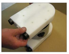
**Fig 23.** Carefully lift on the remaining housing and the stainless steel side plate with booster.
