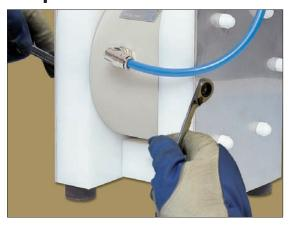
**Fig 1.**First pull out the air hose from the booster to the pump.
