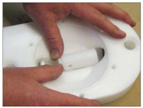
**Fig 16.** Place the spacer sleeve (19) upside down and press it up towards the upper valve seat (20).
