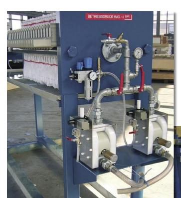
Compact TF filterpress pumps installed for recovering solid waste from water
